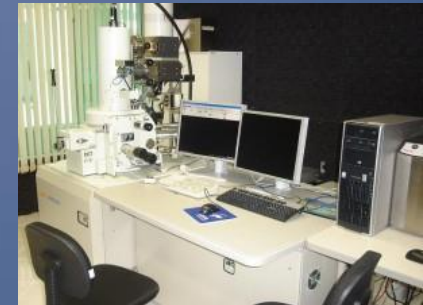
JEOL JSM-6701F Scanning Electron Microscope High resolution: 1 nm (30kV)
