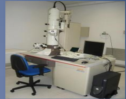
TEM - JEM1011 - Transmission Electronic Microscope , for analysis of organic and biological systems
