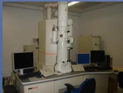
TEM - JEM2100 – Transmission Electronic Microscope, for metal and ceramic materials.
