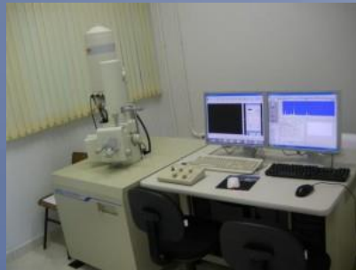
JEOL JSM-6390LV Scanning Electron Microscope with tungsten filament
